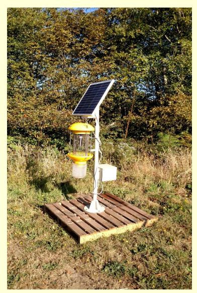
Operates at night using a uv bulb that attracts insects and electrocutes them. It is a self contained unit and is mobile.
