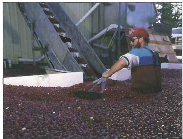
Figure 2.—Using a stepped conveyor belt to move berries from the water into harvest containers.
