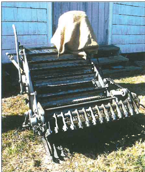
Figure 3.—A Furford dry harvester.
